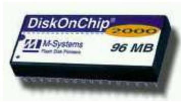
Figure 14: Boitier Disk On Chip
